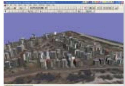
With MapInfo Professional v6.5 came Prism Maps and the ability to create bivariate thematic maps. Extrude regions based on a value or just generate a city landscape view.
